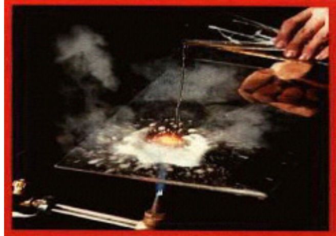
In the photo above, a cutting torch was placed below the ROBAX® and heated until it was red-hot. Cold water was then poured onto the glass from above. There was NO Breakage.
